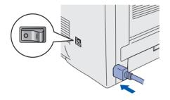
2 Plug the AC power cord into an AC outlet. Turn the power switch on.
